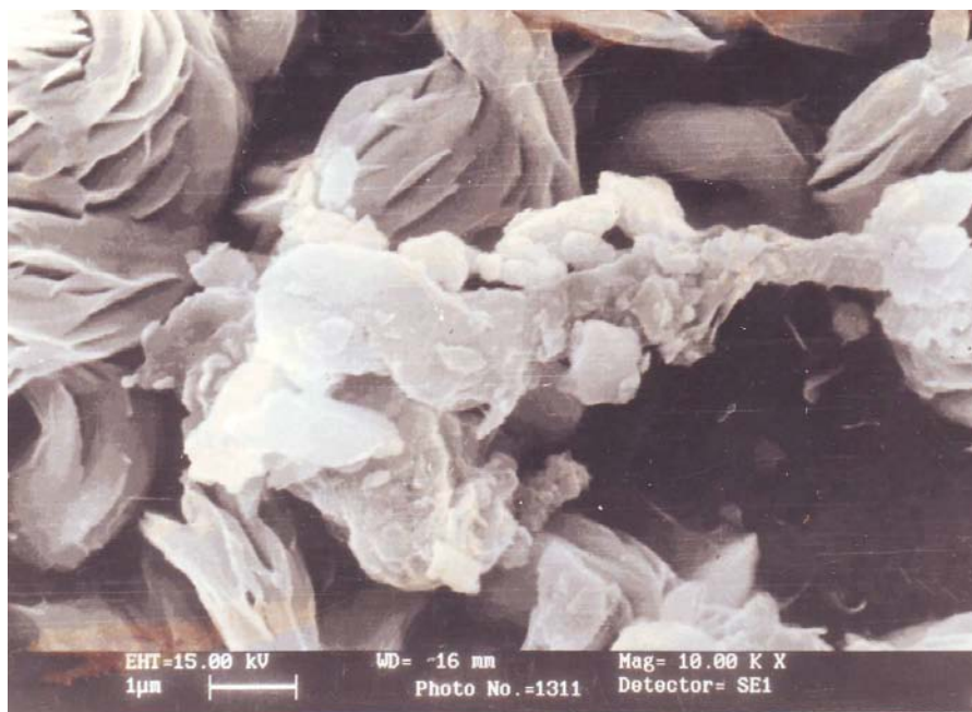
Fig. 3 SEM of annealed CdS film (magnification = 10 k)
