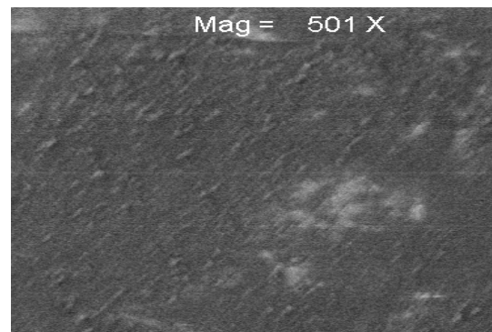
Fig.3b: SEM of film annealed at 373K
